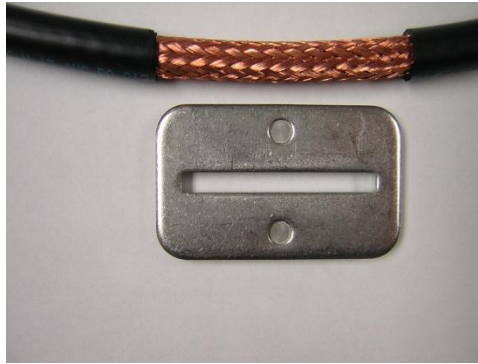
Figure 7 - Remove 2" of Jacket From Coax.
